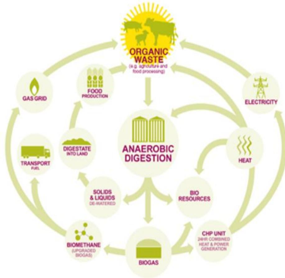
*Multiple products of anaerobic digestion (Modified from ADBA with permission)*
