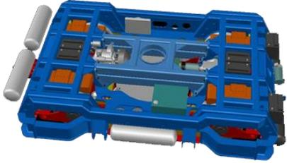
Integrated Bogie Frame with positioned green gas biomethane cylinders
